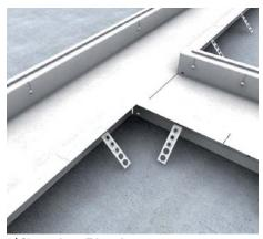
**7** | Shortening a T-junction Push the branch duct bottom piece to the notch, shorten the side profile by 0,3 m and hinge it behind the inward bend.
