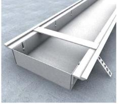
**11 | Spacer** Before applying screed, insert one spacer UBKDB per duct metre. The distance plate is to be removed after the hardening of screed.
