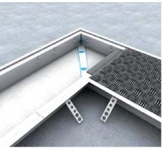
**9** | **T**-junction final assembly Push the branch duct bottom piece to the notch and cut the dummy cover UBKD as well as the profile.
