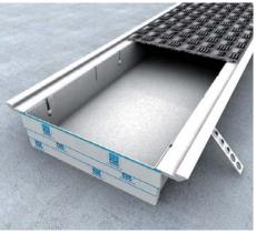
12 | Dummy cover Mask all open areas and insert dummy covers only after the application of screed.
