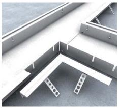
**6** | Inward profile bend In order to create a branch, notch the duct bottom piece as well as the side profile. Then insert two inward profile bends UBKIB.
